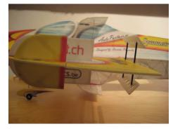
The pictures show the state when flying straight ahead. The attachments above and below the two ailerons have their full braking effect. When the aileron is extended, the effect – as can be seen from the pictures – is reduced. With a fully extended aileron, the braking effect is virtually zero as the "Depron"
