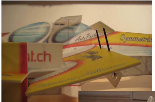
The desired effect of these stabilisers is determined by their size and angle. Their position also plays a part. Michel explains that when searching for the optimum, he cuts out several stabilisers and then tries them out indoors. First he flies without stabilisers, then successively attaches the prepared parts at different locations on the model to achieve overall trim. A great example of practical research and innovation using modest resources.
